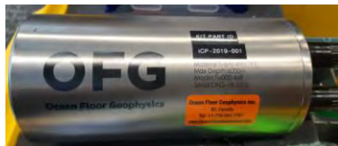
6 channel electric field sensor (redundant X, Y, Z) 100 Hz sample rate
