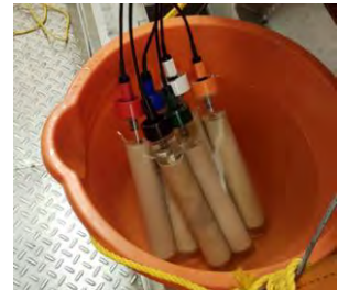
6 low impedance Ag/AgCl electrodes
